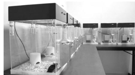
**PhenoTyper** - Video-based observation system for continuous automated monitoring of rodent behavior.
